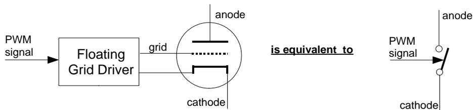
fig.3 – Functional equivalent circuit of a triode driven by a bipolar floating grid driver circuit
