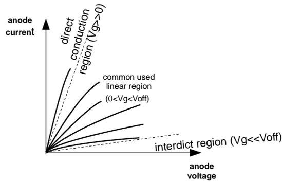
fig.1 – V-I anode figure extended to the positive grid polarization region
