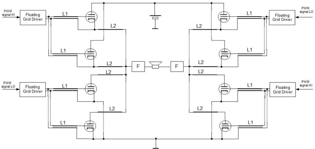
*fig.5 – full bridge class-D power amplifier based on vacuum tubes as switching devices*
