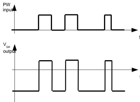
fig.2 – Grid driving by bipolar pulses
