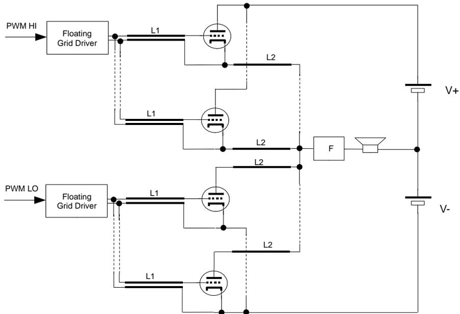
*fig.4 – half bridge class-D power amplifier based on vacuum tubes as switching devices (F output filter, L1, L2 equalized and impedance matched transmission lines)*
